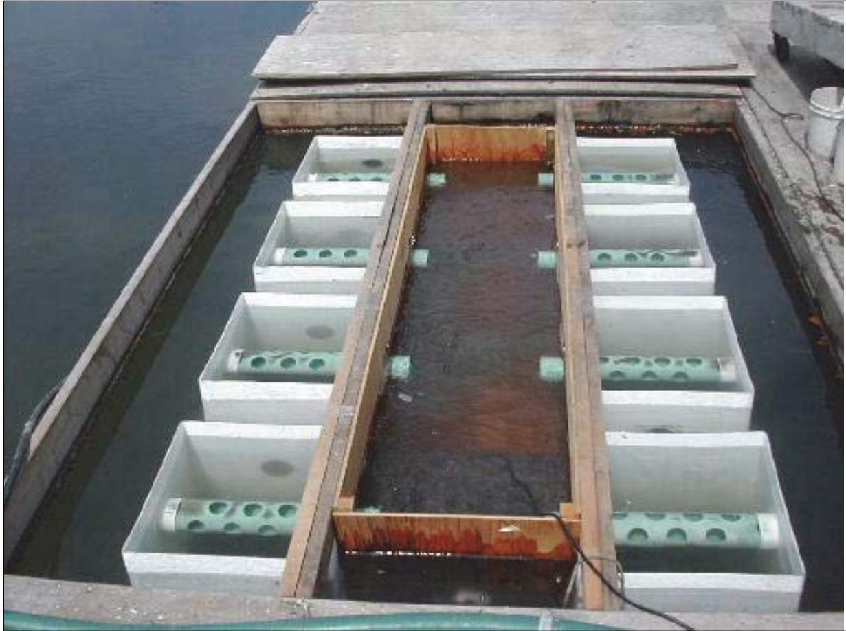
Figure 2. A Floating Upwelling System, or FLUPSY. (Corps 2015, p. 16)
